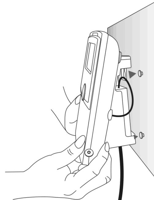
Figure 2-3: attaching the phone to the wall
