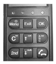
The Function buttons, as shown above, enables the user to enter the menu system of the transceiver and change various settings. Each button is described in detail below. Some of the function buttons have a 2nd function shown in italics at the upper right corner of the function button. To use this 2nd function of a function button, press the "2nd" button and then press the function button.
