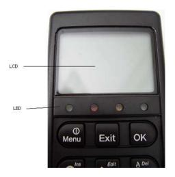
As shown in the picture above, the top of the handset contains the LCD for displaying information to the user. It can be adjusted for contrast and is backlit for viewing in dimly lit areas or night operations. The LCD display is graphically shown below:
