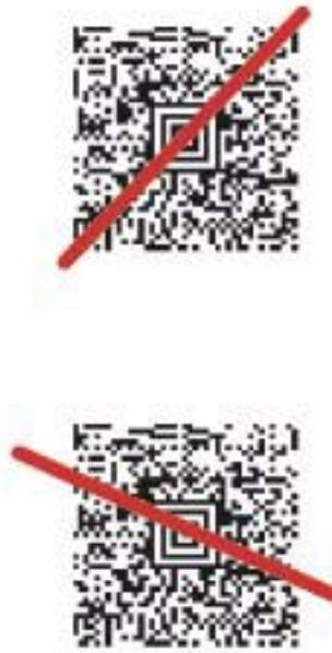
The aiming beam is smaller when the terminal is held closer to the code and larger when it is farther from the code. Symbologies with smaller bars or elements (mil size) should be read closer to the unit. Symbologies with larger bars or elements (mil size) should be read farther from the unit.
