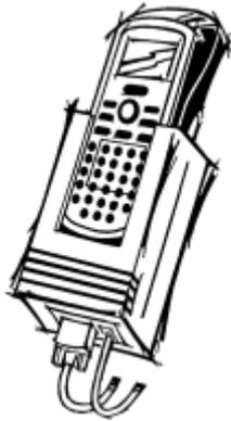
Battery charging and/or communications cradle designed for in-transit applications. Mounted inside a vehicle, this cradle provides connectivity to any RS-232 serial device including printers, radio modems, GPS, on-board computers and vehicle monitoring systems.
