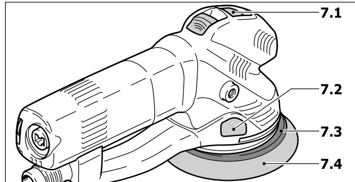
The FastFix system enables tool-free replacement of the sanding pad (7.4):
