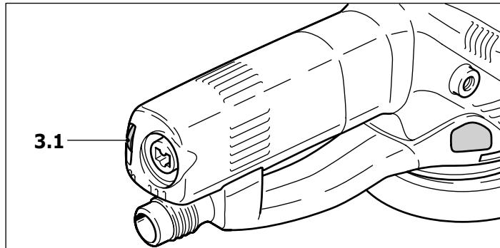
You can regulate the speed steplessly between 3300 and 6800 rpm using the adjusting wheel (3.1). This lets you optimize the sanding speed to suit the material.
