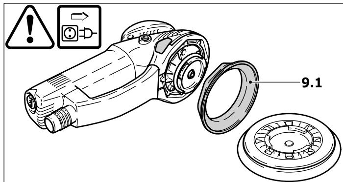
The rubber collar (9.1) prevents the sanding pad from revving up to maximum speed in an uncontrolled manner during eccentric motion (fine sanding). Because the collar wears down in the course of time, it has to be replaced by a new one (order no. 465472) as soon as there is any reduction in the braking effect.
