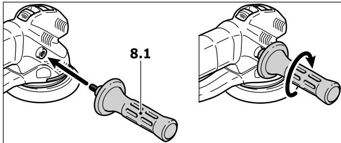
The auxiliary handle (Accessories, 8.1) can be screwed onto either the right or left of the gear head.
