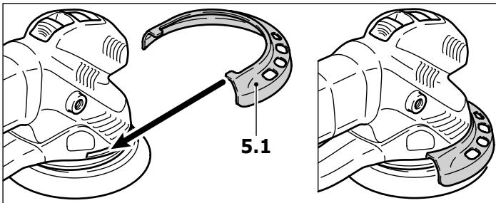
The edge protector (5.1) prevents the sanding pad from touching the edge perpendicular to a surface (e.g. when sanding along a wall), thereby preventing the machine from rebounding.
