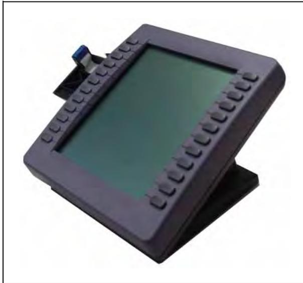
Each KEM has a desk-mount bracket and structural base plate to connect the KEM to an IP Phone 2004 or to another KEM. You can connect a maximum of two KEMs to the IP phone 2004.
