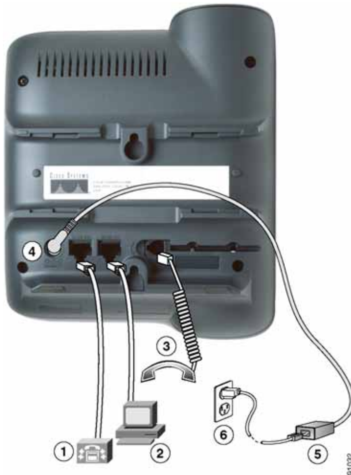
Figure 3-2 Cisco IP Phone Model 7912G Cable Connections
