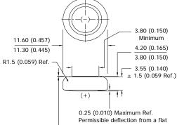
0.13 (0.005) Minimum Ref. (applies to top edge of gasket or edge of crimp, whicever is higher)
