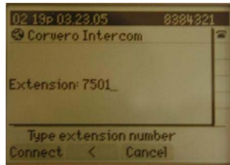
**Step 2:** After you have selected Rapid Broadcast, scroll down or select Option 5. (Corvero Intercom) Type in the extension of the phone you are trying to reach and hit the connect button. After the phone prompts you that your recipient has been contacted, speak into the handset with a very clear voice. **\*\*You can use speakerphone with Intercom but not All – Call.\*\***
