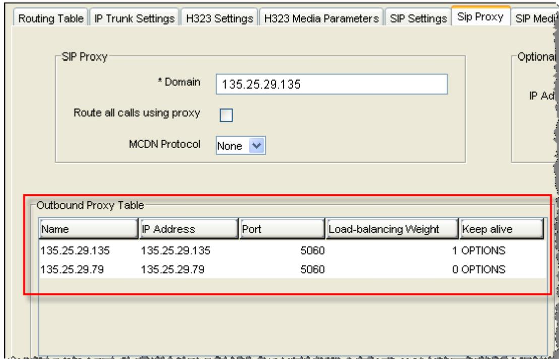
**Figure 15: Outbound Proxy Table for failover to secondary AT&T IPBEs**
