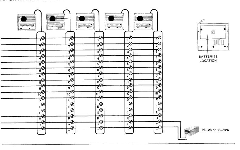
LC-3S WITH SUBSTATIONS V-A, V-B, V-L, OR V-AN
