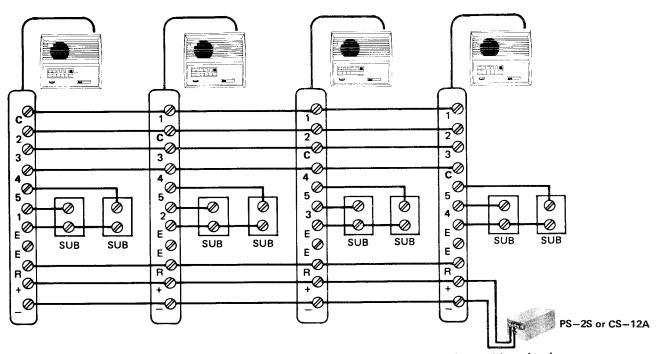
In the above example: (using LC-5S) all master stations can communicate with each other. Substations may call connected master only if the system is not occupied with another conversation.
