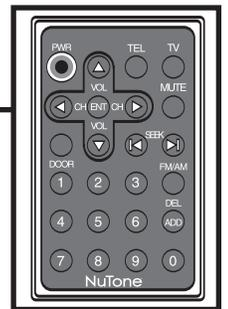
The remote control comes with a disc battery (CR2025) that must be installed prior to operating the remote control.
