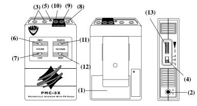
top button again scans to the next FM station. Pressing the **Lower button (12)** resets the FM tuner to 88 MHz. Adjust volume control buttons to volume desired per step four, above. During FM operation, turn the **VOX volume (13)** to a suitable level for Voice Activated Mute to partially lower the FM sound during conversation. If radio operation only is desired, turn the VOX volume all the way to minimum sensitivity.
