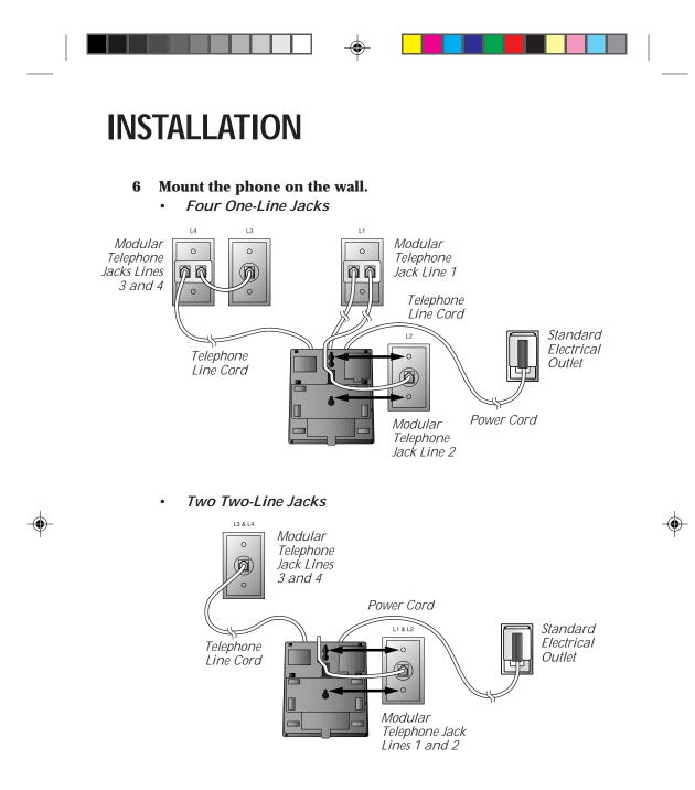
**NOTE:** If you have three modular telephone jacks, mount the phone onto a jack without a wall-mounting adapter. If you have four modular telephone jacks, mount the phone onto a jack without a wall-mounting adapter.
