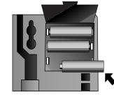
3 Turn the base, as shown, and attach it to the bottom of the phone.
