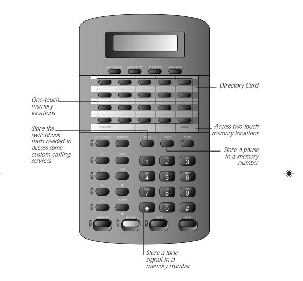
This telephone has 18 one-touch memory locations, and 18 two-touch memory locations. Each location can store up to 16 digits. Dial numbers stored in one-touch locations by lifting the handset (or pressing speaker) and pressing the button for the location. Dial numbers stored in two-touch locations by pressing *LOWER* and the button for the location.
