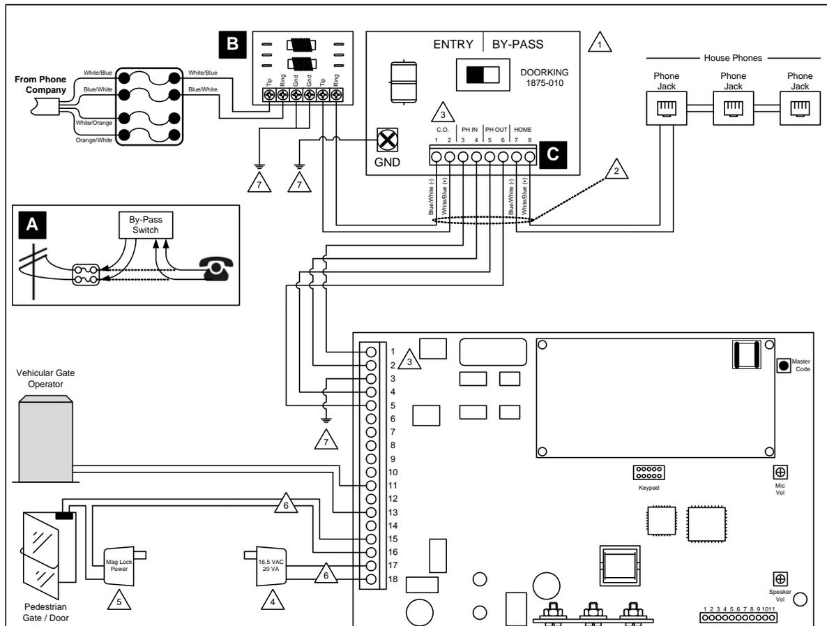
**A** Locate the telephone company demarcation device. **IMPORTANT! Identify the wires that connect to the homeowner's telephones.** Disconnect these wires from the demarcation device and connect them to terminals 7 and 8 on the by-pass switch.
