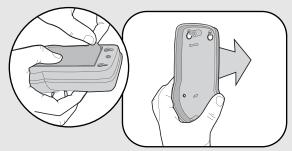
Peel paper from mounting tape. Firmly press intercom onto mounting surface.
