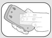
Clean back of intercom and mounting surface using the alcohol wipe.
