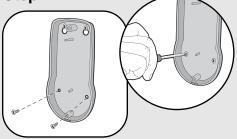
Put the remaining silver screws into the bottom holes of intercom. Tighten screws.
