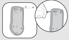
Mount Intercom with small silver screws. See mounting template on page 3. Screw the top two screws halfway into the mounting surface. Place back of intercom over screws. Tighten screws.
