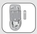
Install 4 AA Alkaline batteries (not provided). (Lithium batteries recommended for colder environments.)
