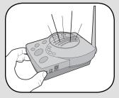
Press the Learn button on the new intercom until a beep is heard. Within 10 seconds put the second intercom into Learn Mode (refer to the following table).
