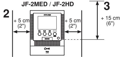
**3** Allow 15 cm (6") or more of vertical open space from the center of the mounting bracket in order to mount the master monitor station and sub monitor station.
