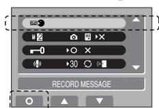
2 In the message recording screen, press CALL button or PLAY button to select the record location. If a message has already been recorded, the selected message is played, enabling you to check the contents of the recording.
