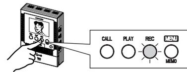
NOTES: 1. Manual recording is not possible during automatic recording (approx. 9 seconds after receiving a call from door station).
