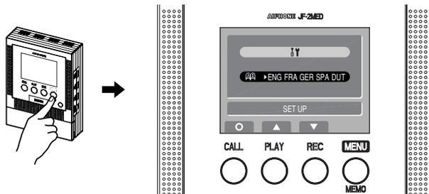
2 Press PLAY button or REC button to select "SET UP", and press CALL button.
