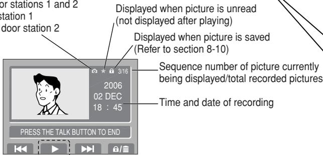
3 To advance the play frame-by-frame, press PLAY button during playback to pause. The play moves forward frame-by-frame each time REC button is pressed. When the frames of 1 picture end, the next picture is displayed.
