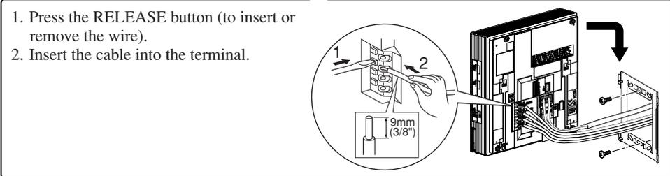
1. Press the RELEASE button (to insert or remove the wire).
