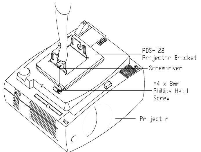
1. Invert the projector and place it on a soft and flat surface. Remove any foot levelers that might possibly prevent the correct installation of the bracket.
