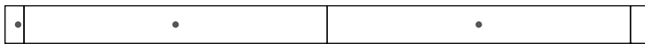
16' Run: 8' (243.84cm) Master Module, 8' (243.84cm) Slave Module, Single Sensor End Set, and Intermediate Cable Assembly.
