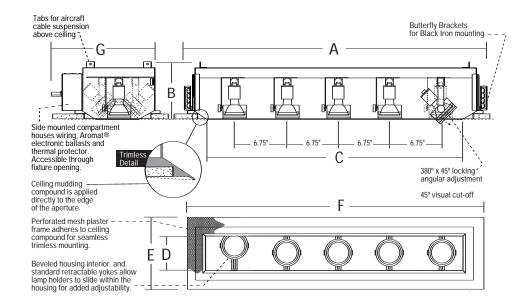
**Includes Aromat® Electronic Metal Halide Ballasts**
