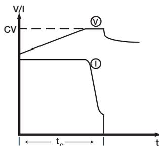
Figure 1. End of Charge Profile
