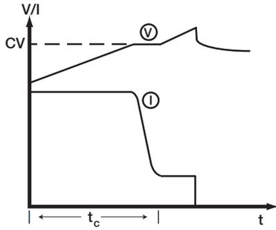
Figure 2. End of Charge Profile with Equalize
