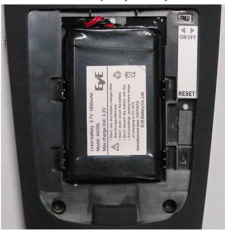
TPMC-4XG-BTP in Battery Compartment of TPMC-4XG-B
