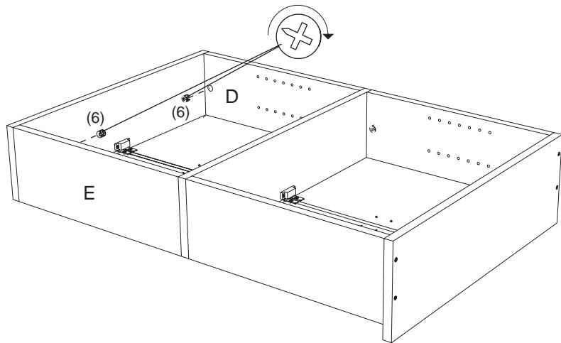
9. Attach panel (C) to unit. Insert CAM locks into panels (D) & (E). Turn CAM locks clockwise to secure.
