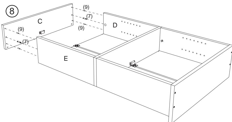
8. Screw in CAM screws (7) in center hole at each side of top panel (C). Insert wood dowels (9) into remaining holes of to panel.
