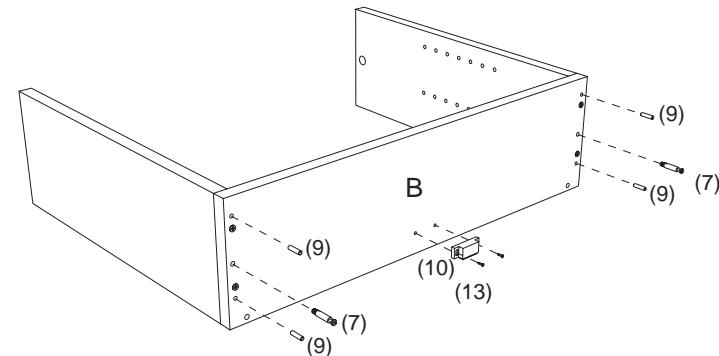
4. Attach magnet (10) to center panel (B) with screws (13). Screw in CAM screw (7) into center hole of each side of panel (B). Insert wood dowels (9) into remaining holes.
