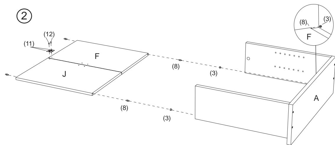
2. Attach metal plates (11) to top corners of doors with screws (12). Insert plastic insert (3) into (A). Insert pins (8) into the hole of doors (J) and (F). Attach door (J) and (F) to panel (A). Pin (8) should fit into plastic insert (3). See Diagram 2A.
