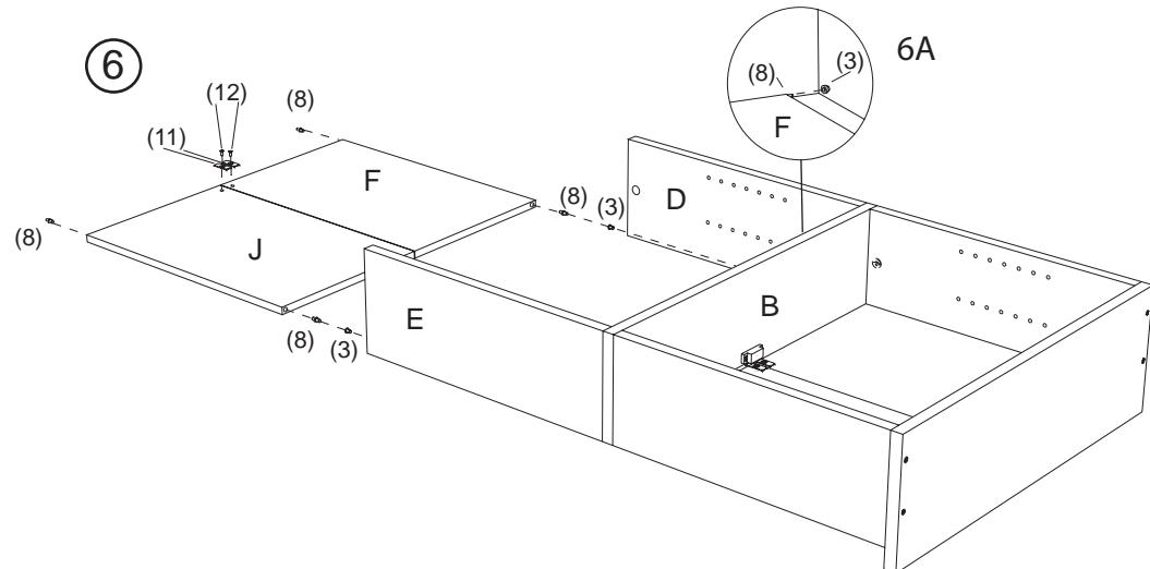
6. Attach metal plates (11) with screws (12) to doors (J) & (F). Insert plastic insert (3) into (B). Insert pins (8) into the hole of doors (J) & (F). Attach doors (J & F) to panel (A). Pin (8) should fit into plastic insert (3). See diagram 6A.
