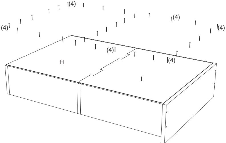
10. Lay backboards (H) & (I) onto the back of the unit. Use a hammer to attach backboards with nails (4).
