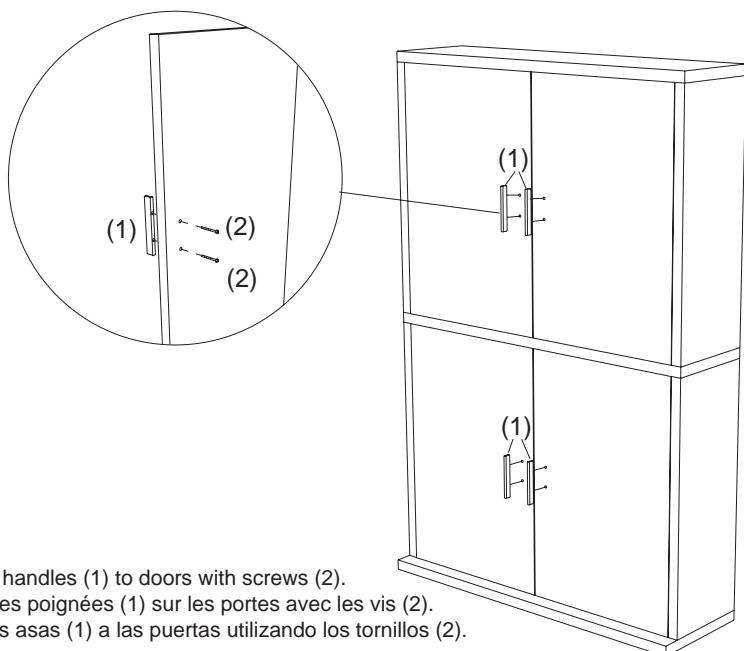
11. Attach handles (1) to doors with screws (2).
