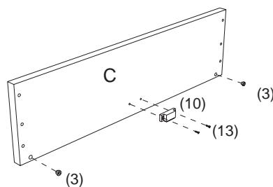
7. Attach magnet (10) to top panel (C) with screws (13). Insert plastic insert (3) into (C).
