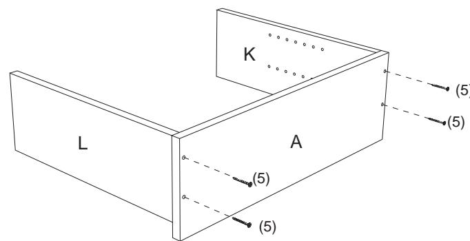
1. Fasten (A) to side panels (L) and (K) with screws (5).
