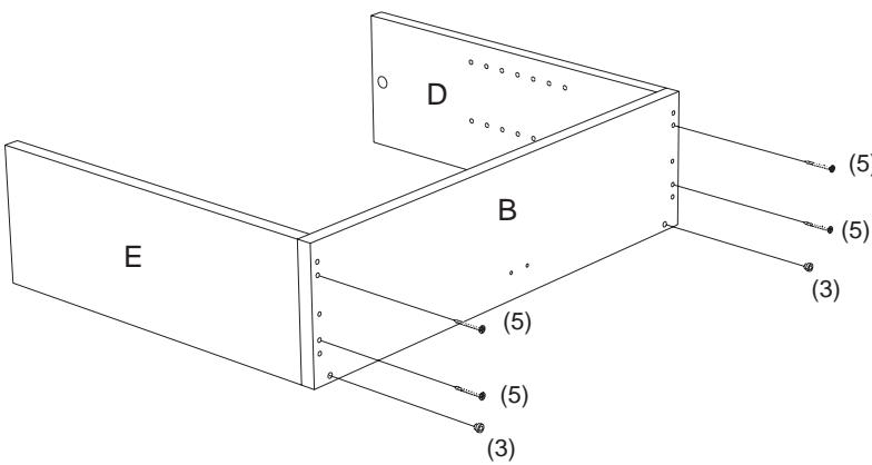
3. Insert plastic insert (3) into (B). Attach center panel (B) to side panels (D) & (E) with screws (5).
