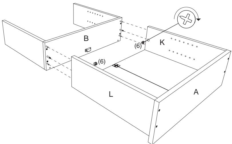
5. Attach top and bottom sections. Insert CAM locks into panels (L) & (K). Turn CAM locks clockwise to secure.
