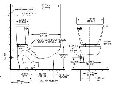
NOTES: THIS TOILET IS DESIGNED TO ROUGH-IN AT A MINIMUM DIMENSION OF 305MM (12") FROM FINISHED WALL TO C/L OF OUTLET. SUPPLY NOT INCLUDED WITH FIXTURE AND MUST BE ORDERED SEPARATELY
