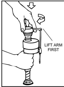
• Replace TOP by engaging lugs and rotating 1/8 turn clockwise. **MAKE CERTAIN TIP IS TURNED TO THE LOCKED POSITION. VALVE MAY NOT TURN ON IF TOP IS NOT FULLY TURNED TO THE LOCKED POSITION.**
