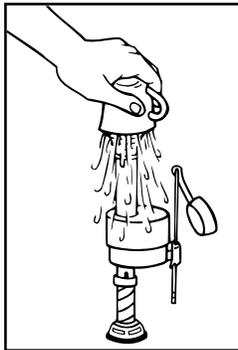
• While holding a container over the uncapped VALVE to prevent splashing, turn water supply on and off a few times. Leave water supply off.
