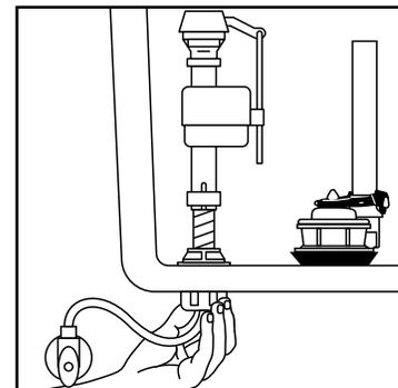
With correct washers in place (see Step 9a), tighten COUPLING NUT 1/4 turn beyond hand tight. DO NOT OVERTIGHTEN.
