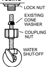
Use existing spiral cone washer. Fluidmaster cone washer may not seal completely on spiral type supply line.
