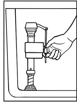
Turn on water supply. Adjust water to desired level by squeezing water level adjustment clip and moving FLOAT CUP up or down along stainless steel link.
