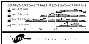
The four profiles on the right side of the console show how the speed and incline of the treadmill will change during the programs. The numbers beside the profiles show the maximum speed and incline settings for the programs.
