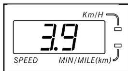
Each time a button is pressed, the speed setting will change by 0.1 mph; if a button is held down, the speed setting will change in increments of 0.5 mph. To change the speed setting quickly, press the OneTouch Speed buttons. **Note: The console can display speed and distance in either miles or kilometers. For simplicity, all instructions in this section refer to miles.**
