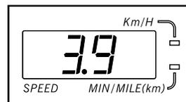
Note: When the Km/H indicator is not lit, the console will display speed and distance in miles; when the Km/H indicator is lit, the console will display speed and distance in kilometers. To change the unit of measurement, first hold down the Stop button while inserting the key into the console. An
