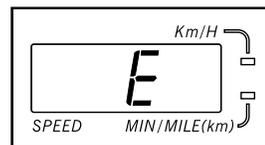
“E” for English miles or an “M” for metric kilometers will appear in the display. Press the Speed  $\Delta$  button to change the unit of measurement. When the desired unit of measurement is selected, remove the key and then reinsert it.
