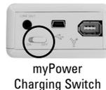
**NOTE:** As myPower charges the iPod battery, the battery capacity in myPower will decrease and each light on myPower will begin to turn off in sequence from right to left. When myPower is completely out of battery, the red light will turn off. At this point, you must charge myPower.
