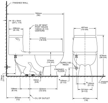
THIS TOILET IS DESIGNED TO ROUGH-IN AT A MINIMUM DIMENSION OF 305MM (12") FROM FINISHED WALL TO C/L OF OUTLET. SUPPLY NOT INCLUDED WITH FIXTURE AND MUST BE ORDERED
