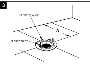
**INSTALL CLOSET BOLTS**Install closet bolts in flange channel, turn 90°, and slide into place 6" (152 mm) apart and parallel to wall.
