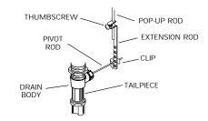
Adjust STOPPER height by repositioning EXTENSION and tightening THUMBSCREW.
