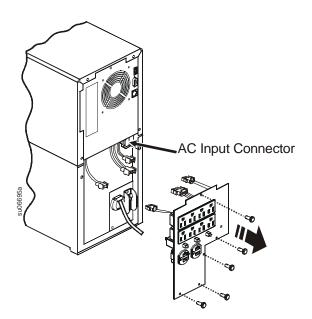
Locate and snap together the corresponding connectors on the UPS and the replacement PDU panel.
