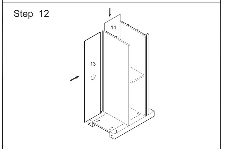
Carefully slide back panels (13,14) into place along the grooves at the back of the frame assembly.
