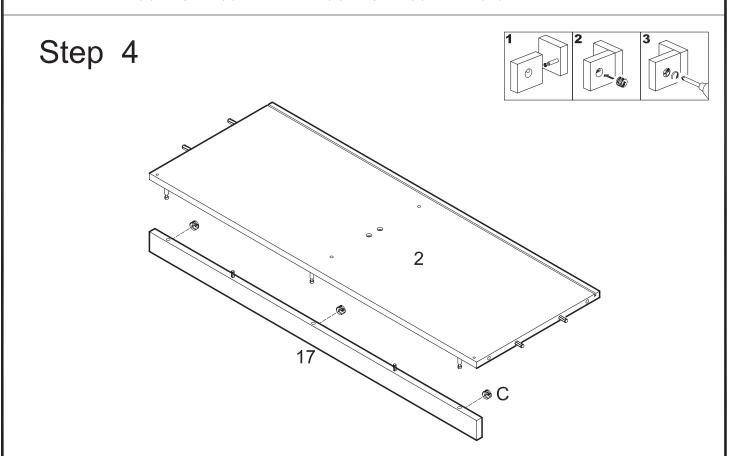
Attach slat (17) to panel (2) using cam bolts and dowels as guides. Insert cam locks (C) into slat (17) and tighten with a screwdriver.
