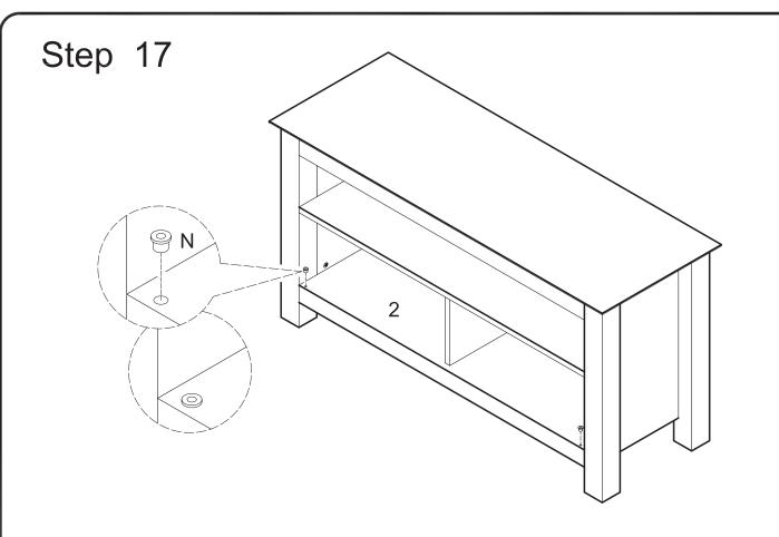
Insert plastic pivots (N) into panel (2).
