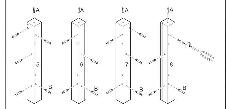
Screw cam bolts (B) into legs (5,6,7,8). Insert dowels (A) into legs (5,6,7,8).
