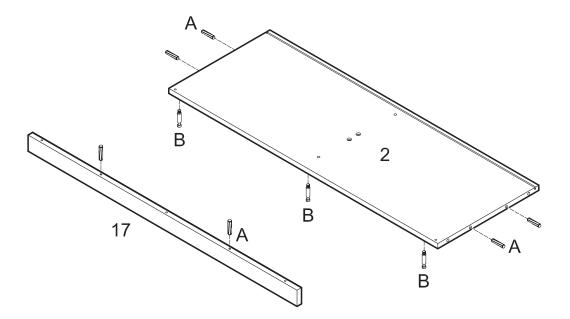
Screw cam bolts (B) into panel (2). Insert dowels (A) into panel (2) and slat (17).
