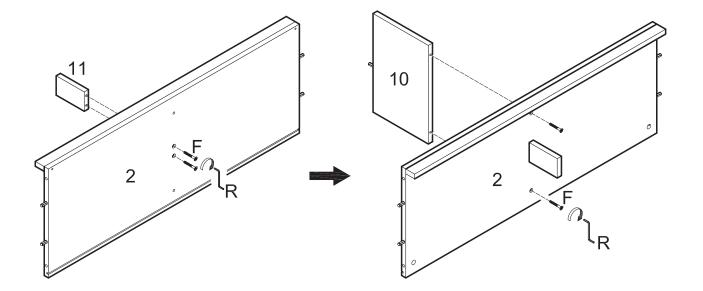
Attach support leg (11) to panel (2) using long bolts (F). Tighten long bolts (F) with wrench (R). Attach panel (10) to panel (2) using long bolts (F). Tighten long bolts (F) with wrench (R).
