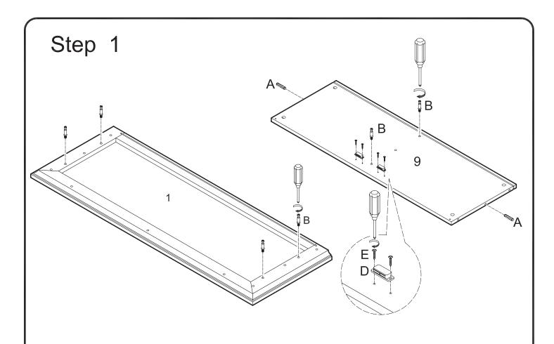
Screw cam bolts (B) into top panel (1) and shelf (9). Insert dowels (A) into shelf (9). Attach door stoppers (D) to shelf (9) using small screws (E).
