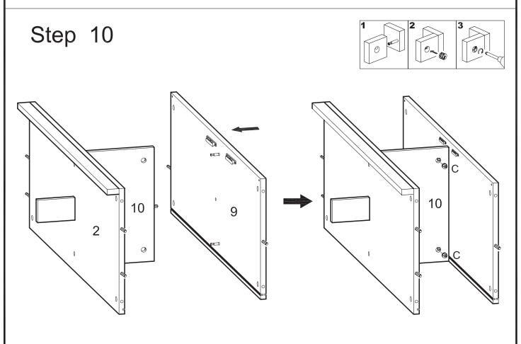
Attach shelf (9) to panel (10) using cam bolts and dowels as guides. Insert cam locks (C) into panel (10) and tighten with a screwdriver.
