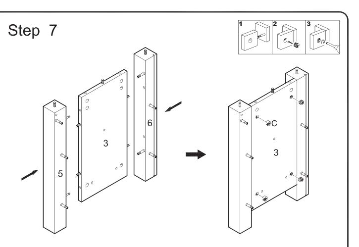
Attach legs (5,6) to panel (3) using cam bolts and dowels as guides. Insert cam locks (C) into panel (3) and tighten with a screwdriver.
