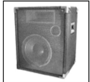
Alpha's Custom P.A. Speakers feature high value and quality performance for portable P.A. systems. Cabinets are a 2-way ported reflex design, carpet covered with pocket handles, stackable interlocking corners, 16 gauge steel grill, dual 1/4" phone jack inputs and constructed of "no void", dimensionally stable structurewood. A high strength polycarbonate stand cup mount, that mates with Ultimate Support speaker stands, is installed flush in the bottom of each cabinet.
