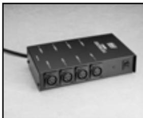
In-line power source for condenser microphones, 9-48VDC, 4 channels, 115v AC source. The CP8506 provides 48V phantom power for up to four microphones. It is a line-powered device that allows the use of remote-powered microphones with systems that do not supply phantom power.
