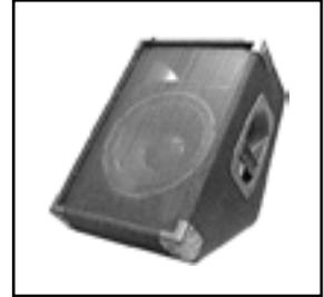
Alpha's Custom Floor Slant Monitors provide exceptional performance and durability. Constructed of 3/4" plywood with a heavy duty 16 gauge steel grill, recessed handles and carpet covering, these monitors are rugged and mobile. This floor monitor has a 12" mid-low driver and 90°x 40°horn; rated 250 watts long term / 500 watts peak power; 8 Ohm nom. impedance; 60Hz-18kHz frequency response. Size: 18.4"H x 15"W x 21"D, 32 lbs.
