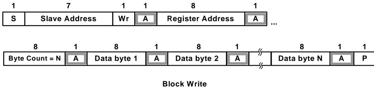
**Figure 4.1 Block Write**
