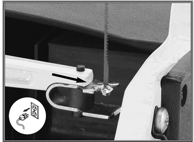
Figure 3. V-notch on lower blade holder.
