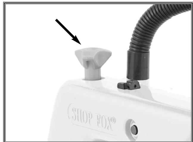
Figure 10. Blade tension knob.
