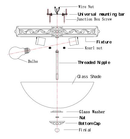
STEP 6: Install the center rod to the fixture;
