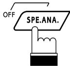
While the main screen for a music source is displayed, press the SPE.ANA. button to turn on the spectrum analyzer mode.
