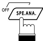
To deactivate the spectrum analyzer mode, press the SPE.ANA. button for at least 2 seconds.
