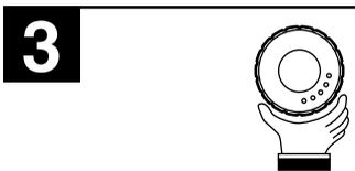
Rotate the rotary encoder and select "DIMMER."
