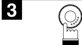
Press the rotary encoder to select "HI LEVEL" or "LOW LEVEL." Each press toggles between "HI LEVEL" and "LOW LEVEL."
