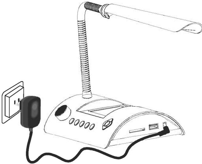
1. Connect the power adapter to the DC IN jack .
