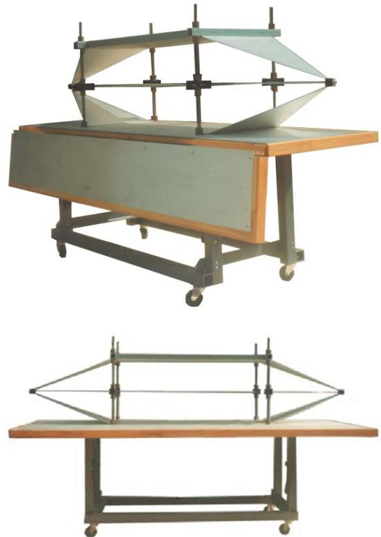
**The TDK RF Solutions TP-02 Triplate and integrated table is specifically designed to generate fields for EMC testing in automotive component test environments.**
