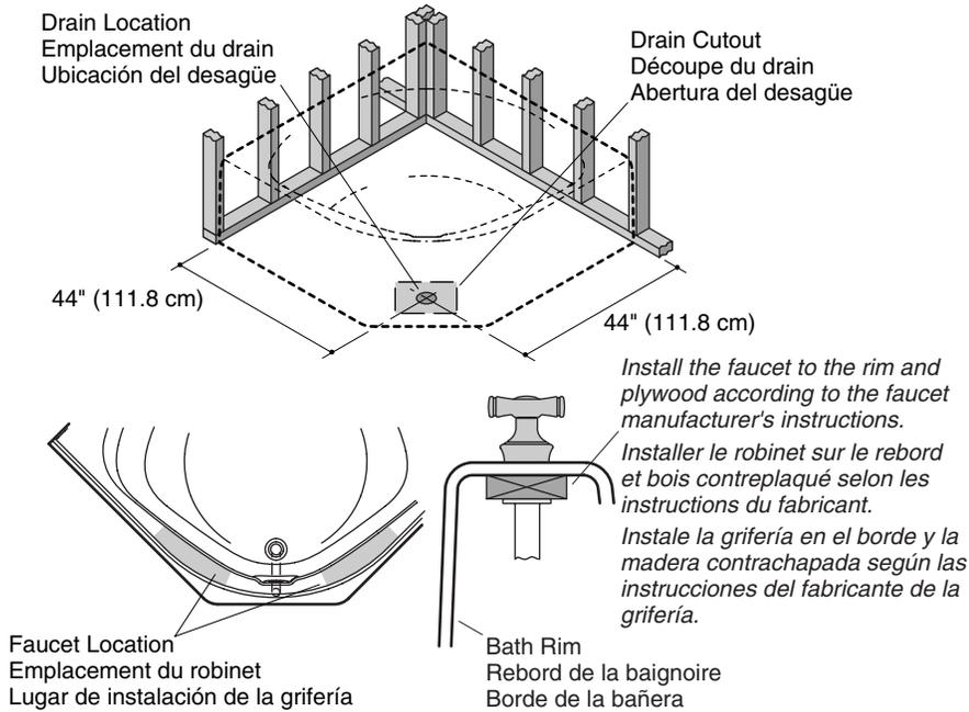
**NOTE:** Provide access to all plumbing connections to simplify future maintenance. Include access at the back of the plumbing wall whenever possible.
