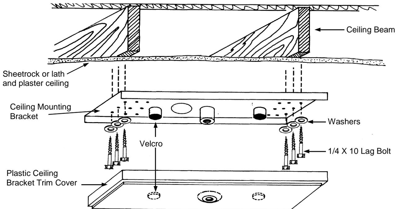
**NOTE: THE OUTER ROW OF HOLES ARE 16" BETWEEN CENTERS WHICH IS THE MOST COMMON BEAM SPACING IN RESIDENTIAL WOOD FRAME CONSTRUCTION.**
