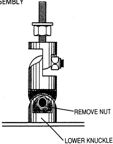
NOTE: PLEASE LOOK OVER THE EXACT MANNER IN WHICH THE POSITIONING ASSEMBLY AND THE ATTACHMENT PLATE GO TOGETHER SO THAT YOU WILL BE ABLE TO REASSEMBLE THEM WHEN YOU HANG THE PROJECTOR.
