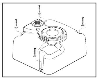
3. Run 5/8" (16mm) I.D. hose to vent fitting and secure with hose clamps.
