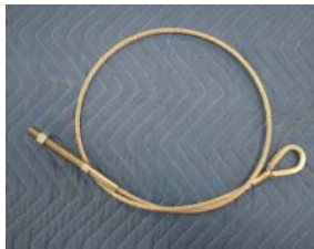
1/4" stainless steel 7 x 19 wire rope assembly w/ 1/2" - 20 NF stainless steel threaded stud with 3-1/2" thread min. on one end only
