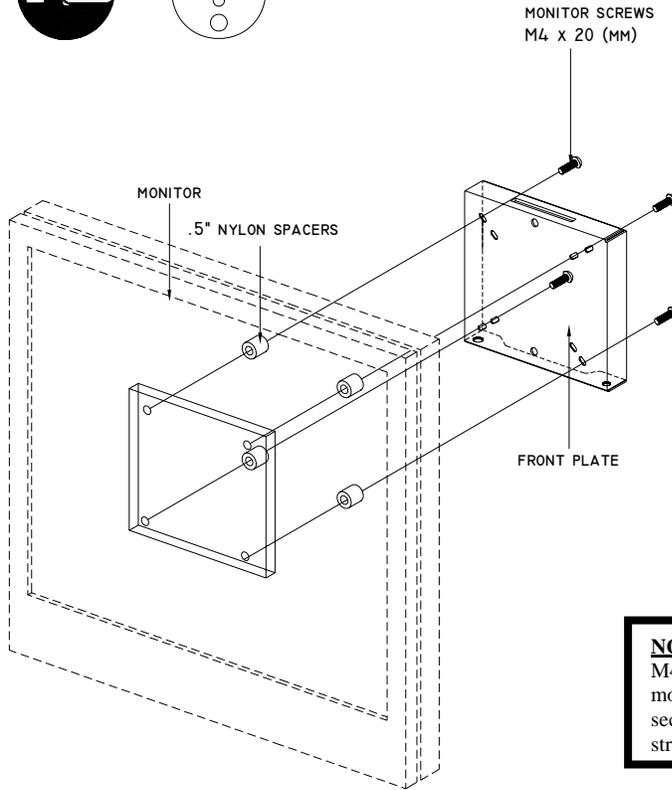
**NOTE:** Use the four (4) .5" nylon spacers and four (4) M4 x 20 (mm) if you have a recessed VESA 75 monitor to compensate for the indentation. Then secure both plates as shown on single stud or solid structure diagrams.
