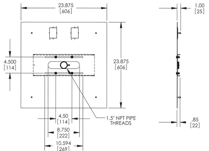
Dimensions are in inches and millimeters [mm].
