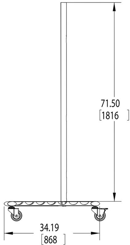
Dimensions are in inches and millimeters [mm].
