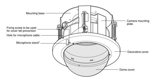
\* If a microphone is used, mount the microphone on the rubber-made microphone stand. Unless the microphone is used, cut the rubber with a nipper or conduct another treatment.
