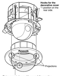
Fixing screw to be used for cover fall prevention
