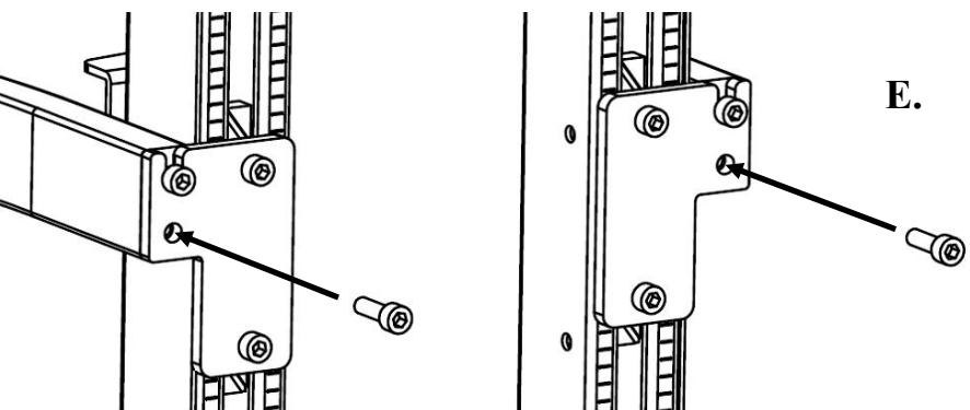
**C.** Insert a **Shelf Screw** into each of the **Shelf's** top screw holes.
