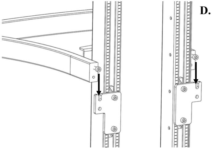
**E.** Tighten the top **Shelf Screw**, then insert and tighten another **Shelf Screw** into the bottom hole.
