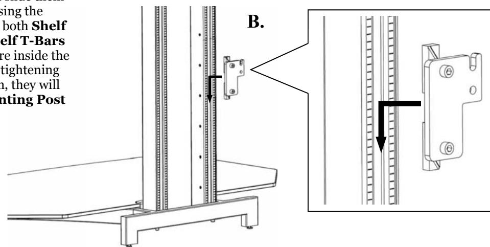
**NOTE:** Ensure that the **Shelf Bracket** is installed with the notched hole on top and facing the outside.
