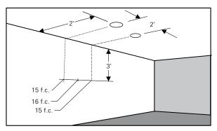
EXAMPLE: 18w with multiple clear reflector units located 2' from wall and spaced 3' on center, the illumination on the wall 3' down from ceiling will be 15 f.c. beneath units and 16 f.c. between units.
