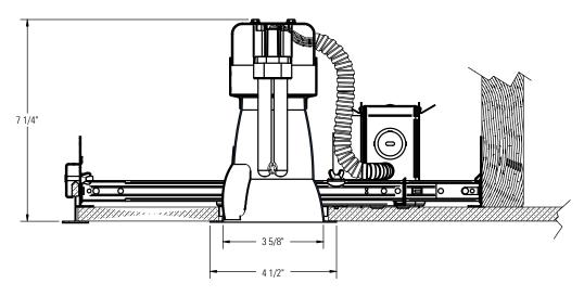
Complete Fixture consists of Frame-In Kit and Reflector Trim. Select each separately.
