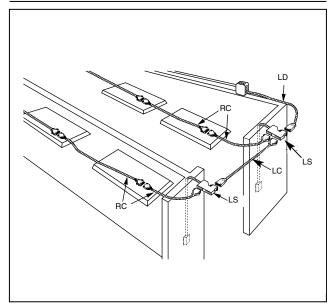
Pre-fabricated distribution cables replace conventional conduit and wire to distribute branch lighting circuits from a junction box. Optional components to the lighting interface.
